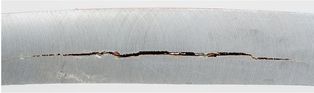
Figure 9: Example of hydrogen embrittlement 51 .
