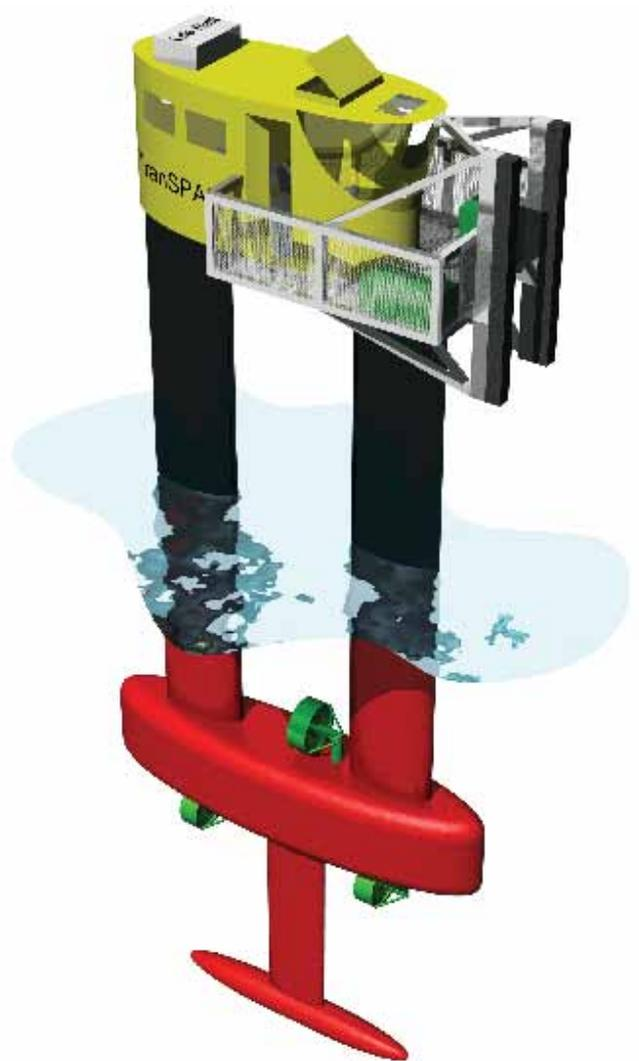
30% over vessels that are currently available. By enabling safe transfers at 3 meters, the propelled spar vessel is expected to increase access time to 310 days per year from 200 days per year currently.
